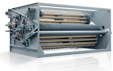
Retrofit module for picking machine WSZ with vertical picker
